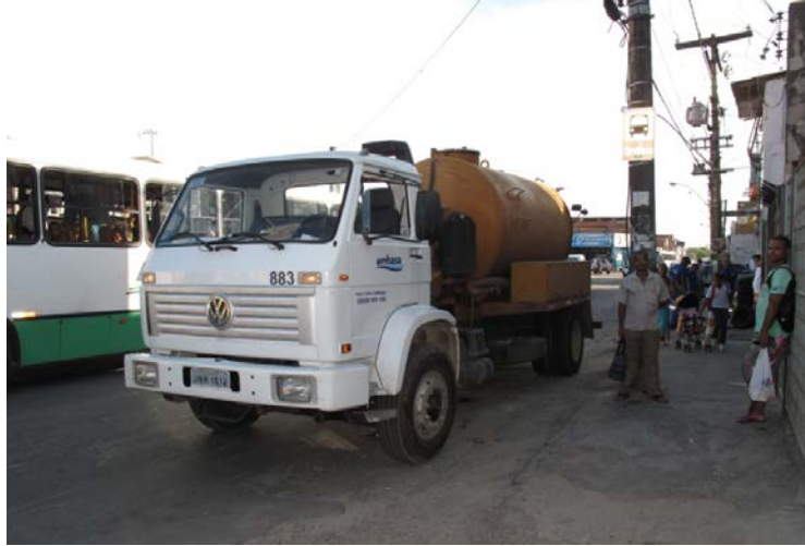
Photo 10. EMBASA's high-pressure sewer cleaning truck used to remove major blockages on the sewer
