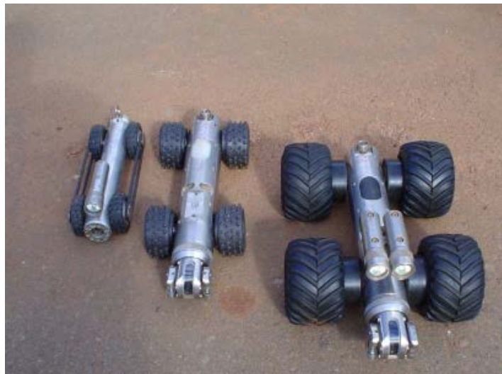
Photo 11. Left: a portable high-pressure sewer cleaner used by CAESB in Brasilia. Right: robots with sewer inspection cameras suitable for sewer pipes of different diameters (source: CAESB)
