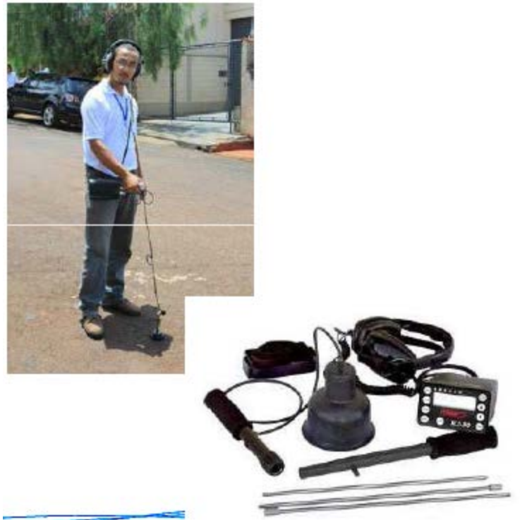
Photo 12. Leak detection equipment used to identify invisible leaks on sewer schemes in Brasília (source: CAESB)
