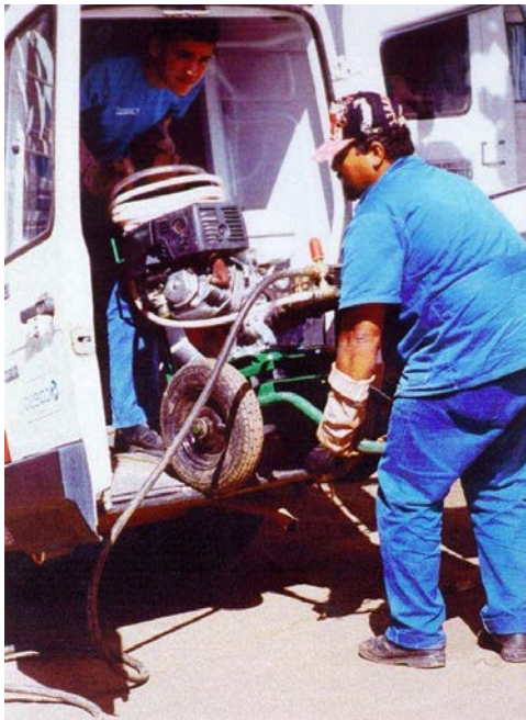
Photo 11. Left: a portable high-pressure sewer cleaner used by CAESB in Brasilia. Right: robots with sewer inspection cameras suitable for sewer pipes of different diameters (source: CAESB)
