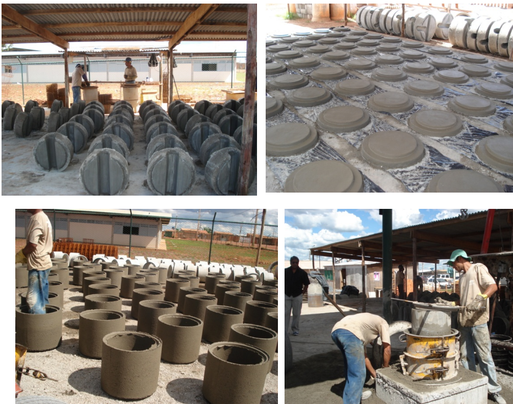
Photo 4. Mass production of 'simplified' manholes in Brasilia (source: CAESB)
